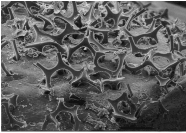
Figure 2 SEM photomicrograph of the “capsule” tissue around a polyurethane (PUR)-coated silicone breast prosthesis. This method demonstrates clearly that the PUR coating has been separated from the prosthesis. The figure shows sub-millimetre “spicules” of PUR embedded in a fibrous connective tissue matrix.
